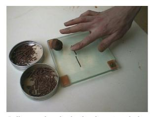
Rolling out threads of soil to determine whether they crumble beyond a particular moisture content is at best crude and of limited reliability. Any notion of 'accuracy' is mute given the changes in structure and mineralogy over just a few metres in the ground. We simply need to know if the soil undergoes volumetric change in relation to its moisture content and the LL test is more reliable and sufficient for our needs.
