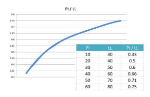
Where we simply need to understand that the soil is a shrinkable clay and setting aside using the Atterberg indices as a means of correlating with the Mc to determine desiccation, the LL alone should suffice.
