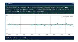
Data is available from 1992 to 2000 and includes velocity, season, area, height, coherence and a range of standard deviations. Ground displacements are shown as a row of dots with movement in mm.
